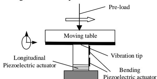
Figure 12 Ultrasonic linear piezo motor
