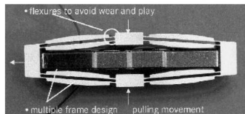
Figure 4 Flexure amplifier structure
