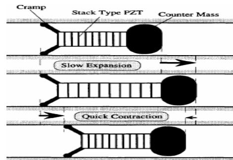
**Figure 9** Principle of inertial drive with piezo
