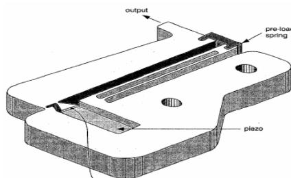
Figure 3 Piezo actuator with lever amplifier
