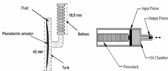
**Figure 7** Hydraulic amplification mechanisms
