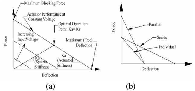
Figure 2 Force vs. deflection of piezo actuators
