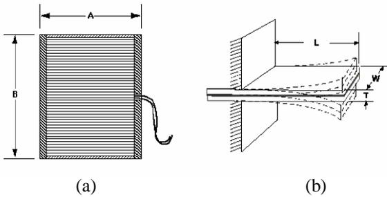
Figure 1 The structures of the stack (a) and bender (b) actuators.
