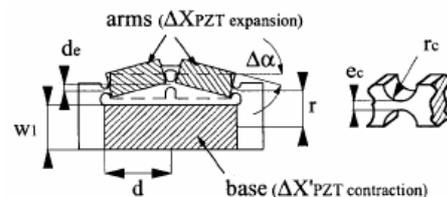
Figure 5 Monolithic piezo actuator
