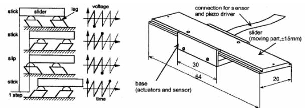
**Figure 10** Stick and slip actuator
