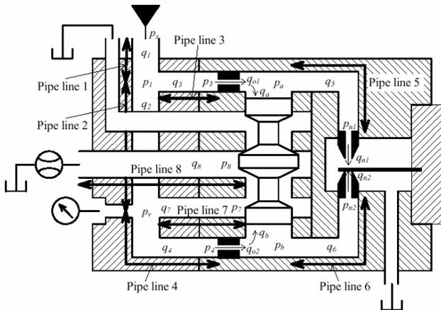
**Figure 8** A 2 stage piezo actuated pneumatic valve.
